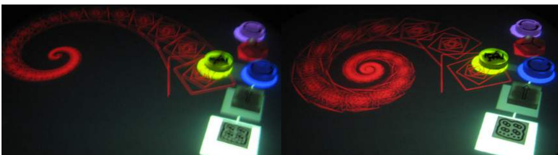
Figure 3.16: A TurTan program using a sinusoidal modifier to dynamically change the parameter of a rotate instruction of a spiral.
