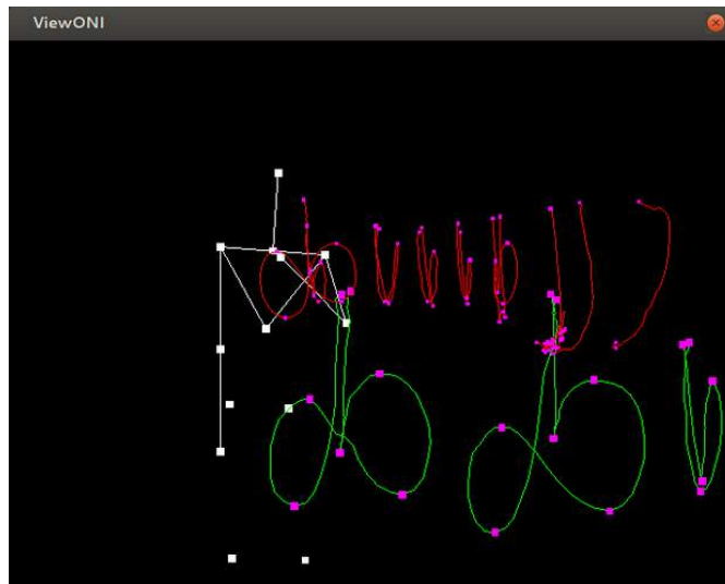
Figure 5.20: Program recognizing valid gestures from Kinect recordings.
