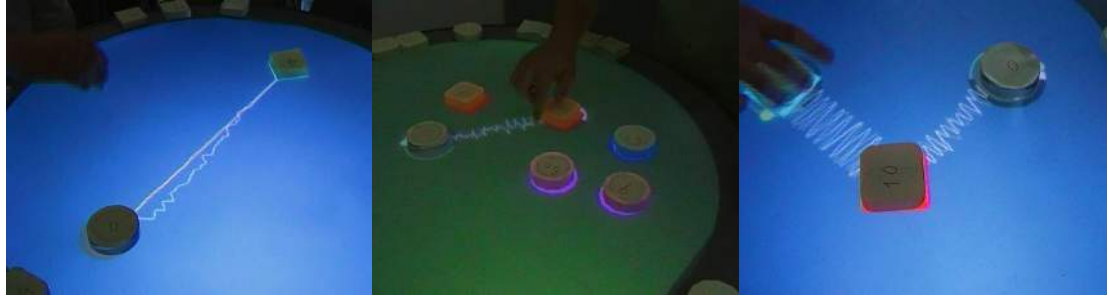
Figure 4.14: Free project results: (a) a Karplus-Strong generator, (b) a MIDI controller and (c) a band-pass filter.
